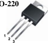
1. Gate 2. Drain 3. Source
